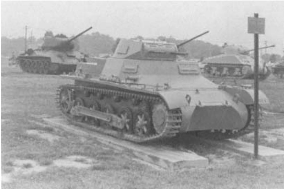
The Panzer I, a light tank mounting only machine guns, was one of the first tanks of the new German Army. Because of the terms of Versailles it was developed under the fiction of producing tractors.
