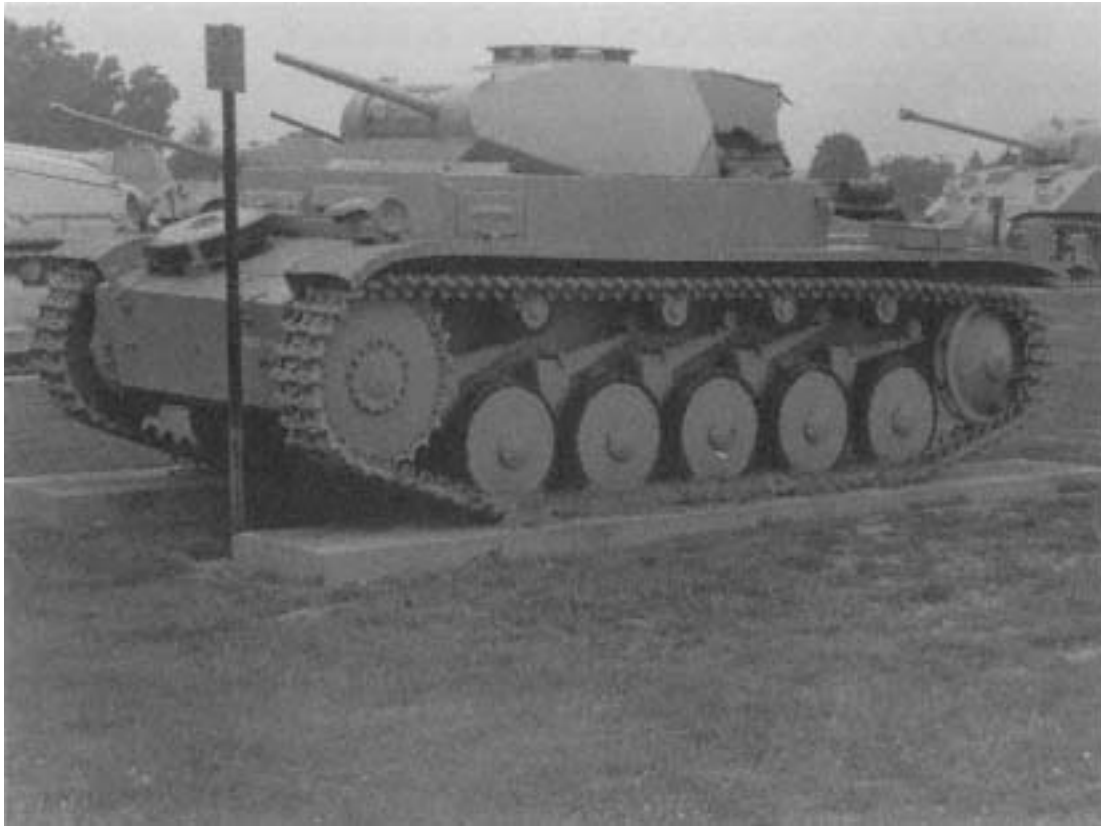
Mounting a 20mm gun, the Panzer II was faster and better armed than the Panzer I. It was obsolete by the 1940 campaign, however.
