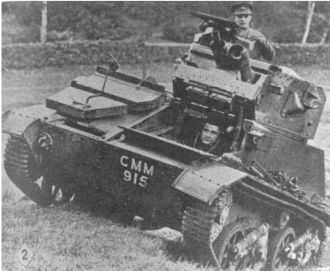
British Mark VI light tanks proved of little use when faced against better armed and armored German vehicles. During the war in France, the Mark VI served as a command and reconnaissance vehicle.
