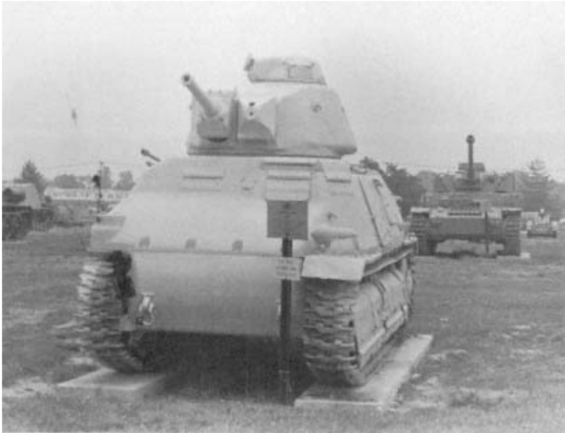
The SOMUA 35 was one of the better tanks of the early war period. Mounting a high velocity 47mm gun and heavily armored, it was a match for the best German tanks.
